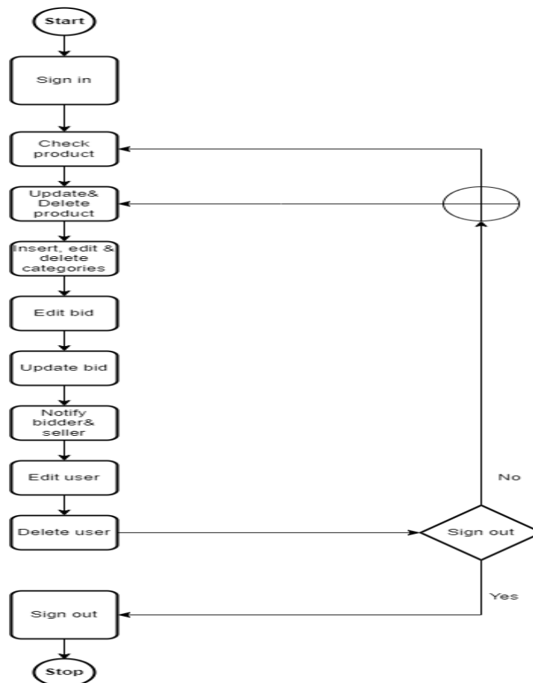
Fig. 3. Flow diagram for the admin panel
